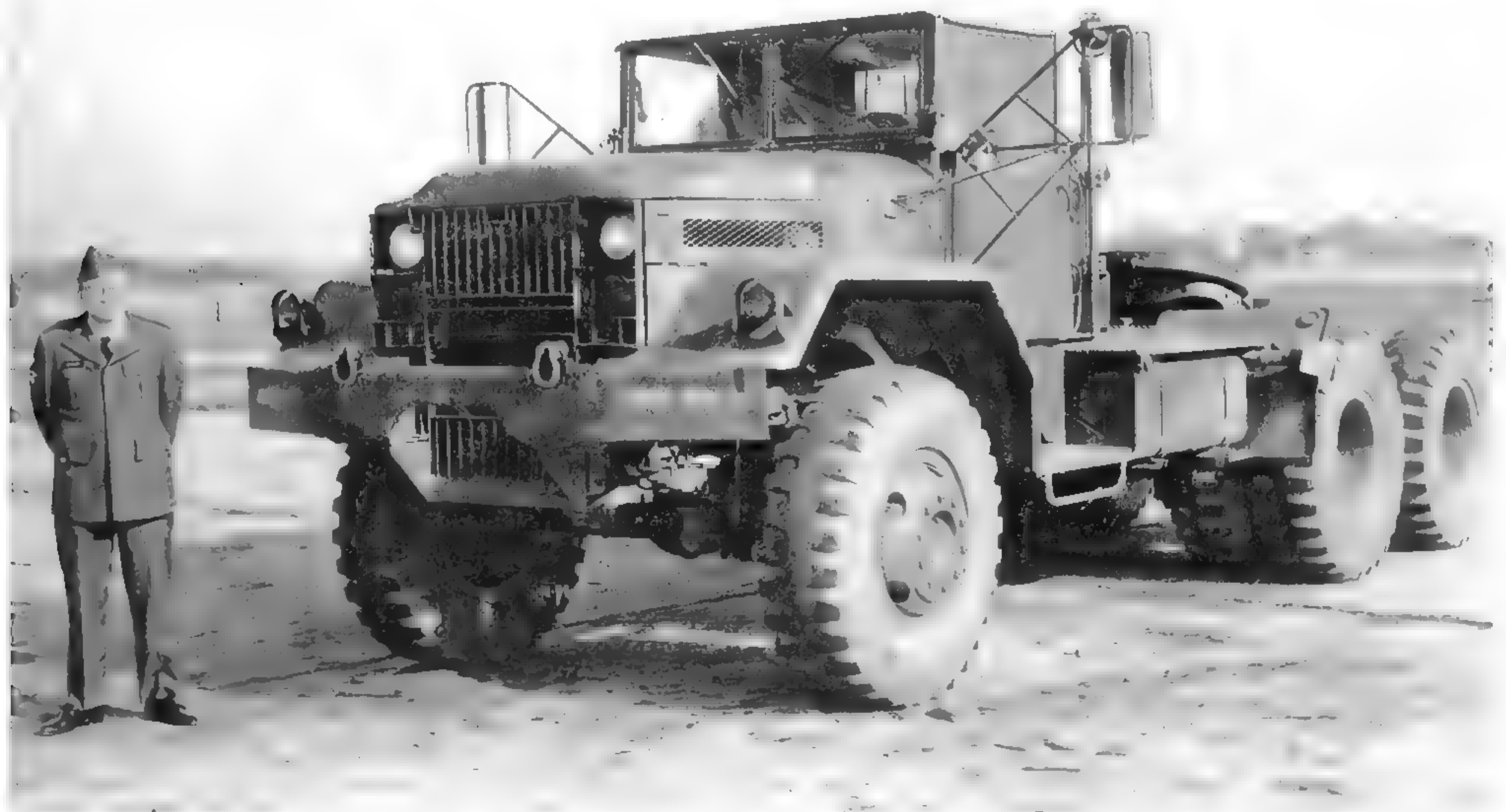
This soldier is dwarfed by the M123C being tested at Aberdeen Proving Ground. Later models added a hinged step in the center of the front bumper to provide access to the engine. The M123C had only a single rear winch. (U.S. Army photo)
